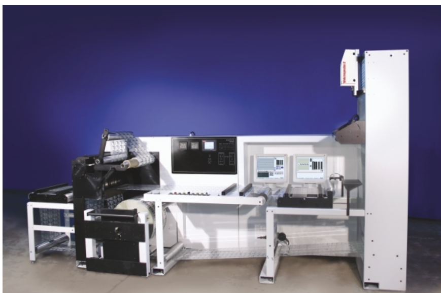
Rewinder with high-resolution Web:Inspector:2 and accumulator for re-inspection of pharmaceutical labels.
